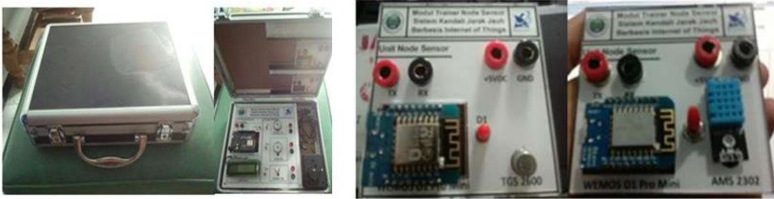
Fig. 10. Remote Control Trainer Based on IoT Kit and Node Sensor Modul Kit
