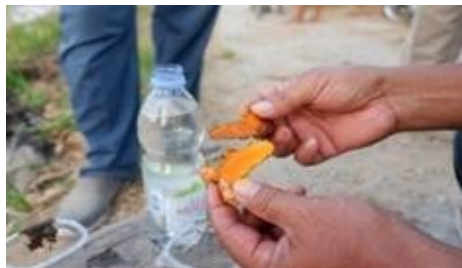
Figure 5. Soil acidity test with turmeric in Suyudan village
