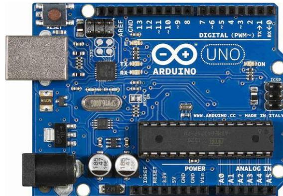
Gambar 1 Arduino UNO Board
